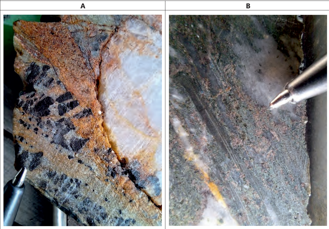
Figure 10-7 Mineralisation in KBDD002: A) Black cassiterite and B) Pinkish cassiterite
