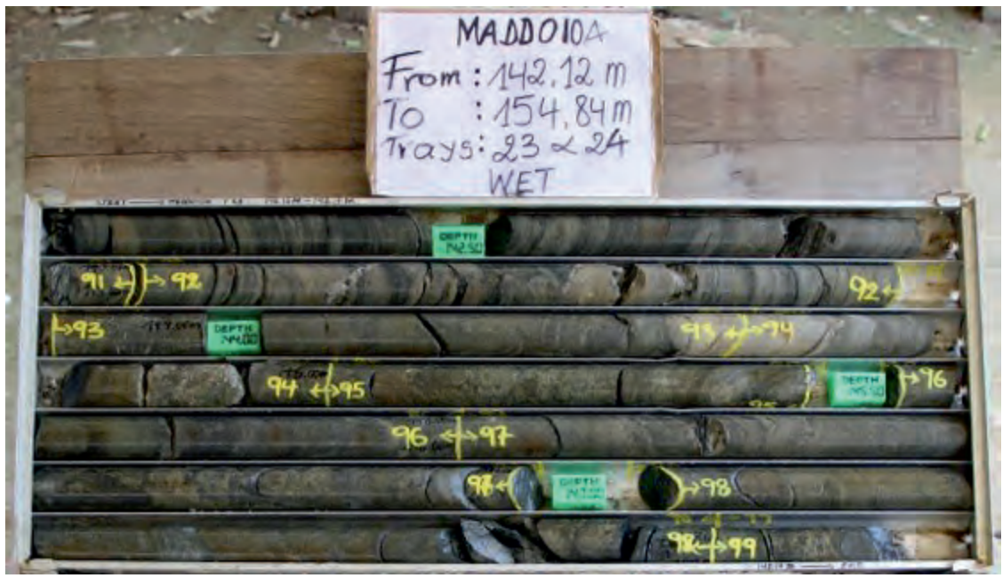
Figure 10-13 Core photo of MADD010A showing pyrite-chalcopyrite dominant massive and semi-massive sulphides.
