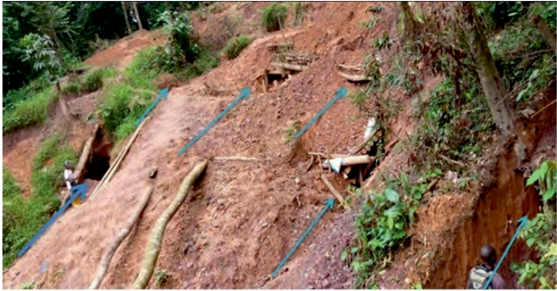
Figure 7-2 Parallel quartz vein sets observed around artisanal workings at Kalayi Boeing
