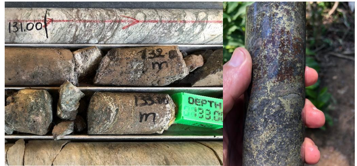
Massive sphalerite (zinc) in drill core (left) & high grade chalcopyrite (copper) (right) at Mont Agoma
