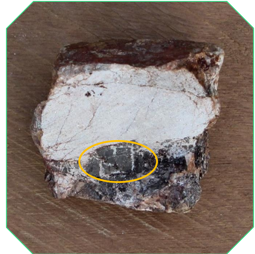
Visible cassiterite in drill core at Kalayi
