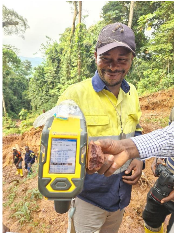
Figure 5: Niton Reading (17% Sn) of Tin Ore being Mined by Artisanals at Kalayi. Note: Strongly Hematized Ore from Oxidation of Chlorite
